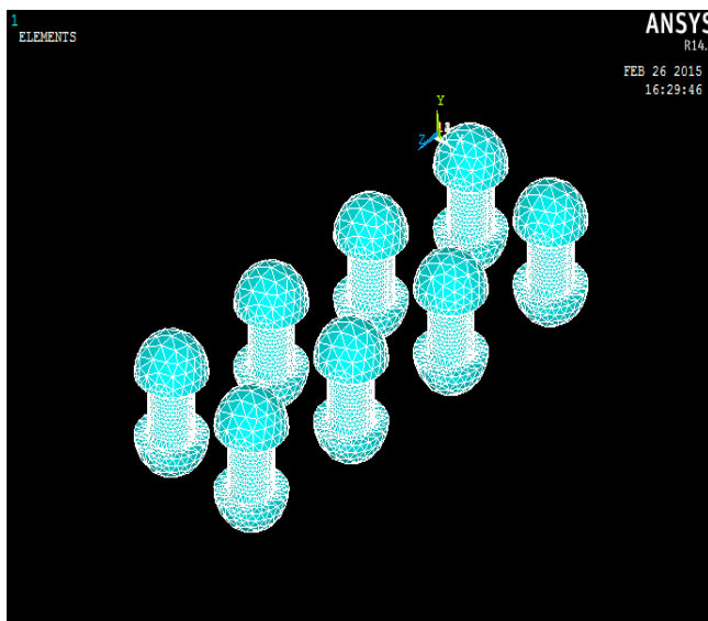
Fig. 4: Finite element mesh of rivets
